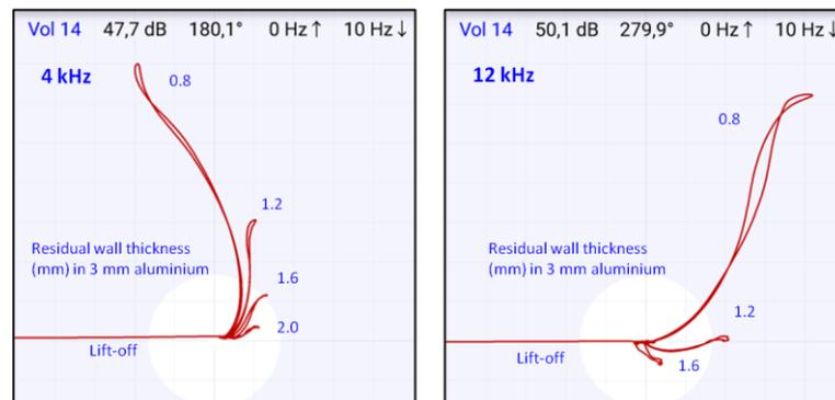
**Figure 3. Wall reduction in aluminium: Left: At 4 kHz all reductions are well detectable. The phase spreading is mediocre. Right: At 12 kHz the phase spreading is significantly better but due to lower penetration not all reductions can be detected.**
