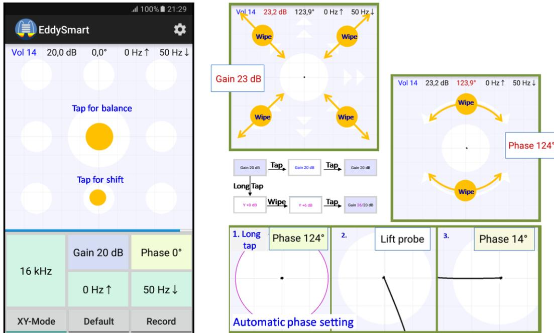
**Figure 4. Left: Balancing and offset may be adjusted by tapping dedicated areas in the xy-plane. Right: Gain and phase are set by wipe gestures on the screen. Automatic lift-off setting will be initiated by long tap on the phase button. While lifting the probe the flying dot crosses the phase circle and the phase is turned accordingly.**
