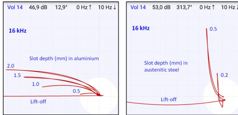
**Figure 2. Surface crack inspection: Left: Slots of different depth in aluminium simulate surface cracks in highly conductive material. Right: Slots in austenitic steel represent cracks in poorly conductive but slightly ferromagnetic material.**
