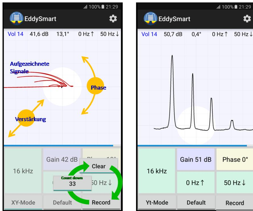
Figure 6. Left: The recorded signals may be manipulated afterwards for best visibility. Right: In yt-mode the time variation of the y component is shown.
