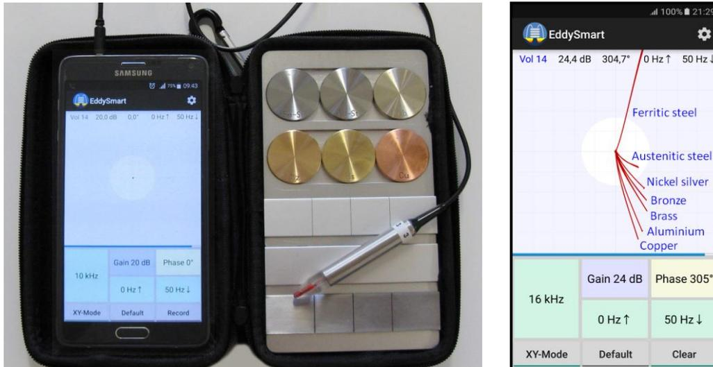
**Figure 1. Left: EddySmart kit consisting of the Smartphone (Galaxy Note 4), the reference set and an absolute probe. Right: Eddy current signals of different materials in the xy-plane on the smartphone screen.**
