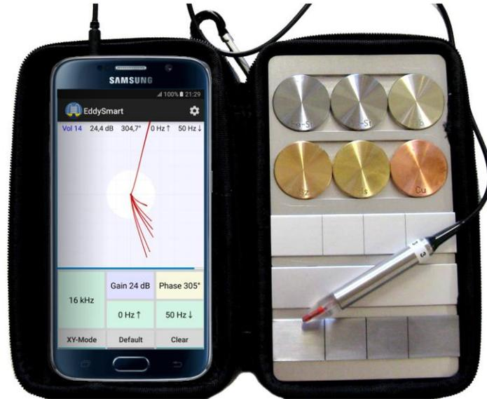
**Figure 1. Smartphone as eddy current instrument. The kit contains a probe and reference pieces for many eddy current inspection tasks.**
